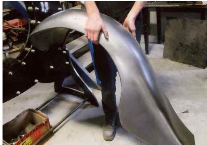
*Left hand rear mudguard made for Ford V8*
